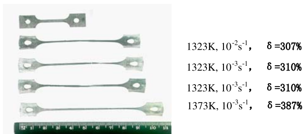
Fig. 1 Macrographs of fracture specimens of NiAl–28Cr–6 Mo alloy
